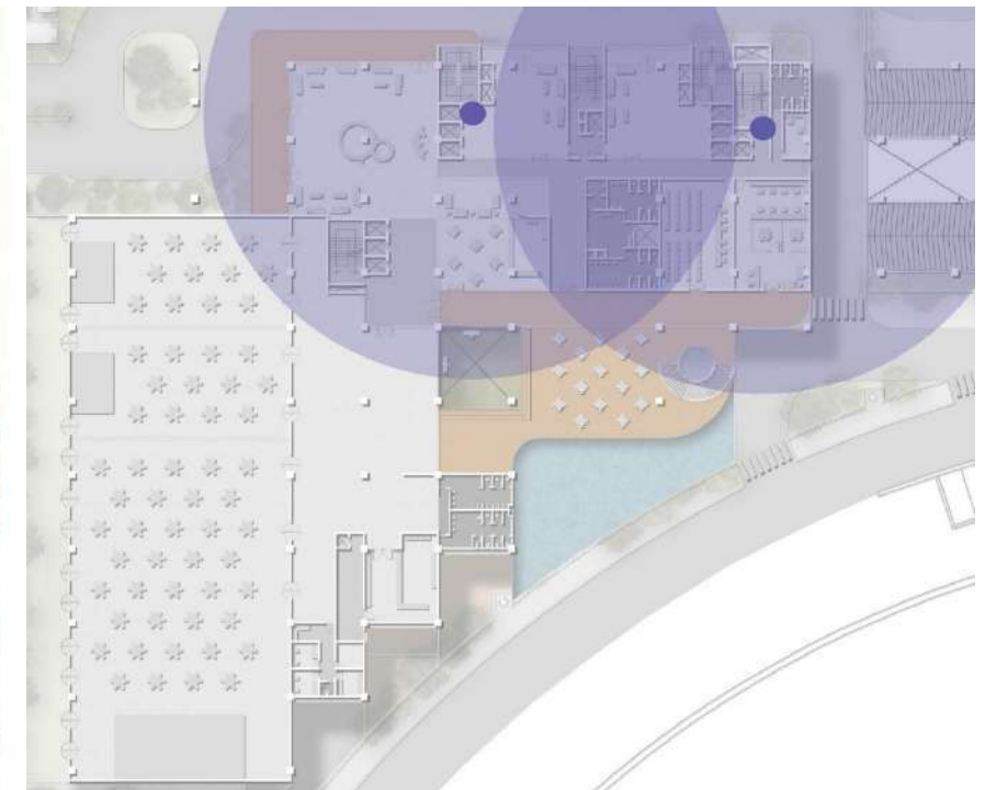
FIRE SAFETY: 30.0 M RADIUS FROM SERVICE CORES
