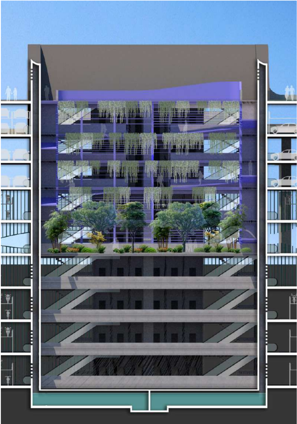
SECTION THROUGH THE WIND CATCHERS/COOLING TOWERS
