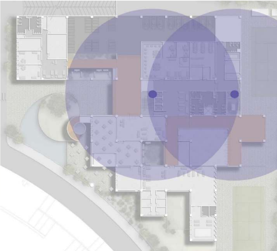
FIRE SAFETY: 30.0 M RADIUS FROM SERVICE CORES
