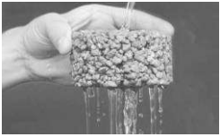
Permeable Asphalt/Porous Concrete Used in vehicular paths; maintains functionality with water percolation; Promotes groundwater recharge
