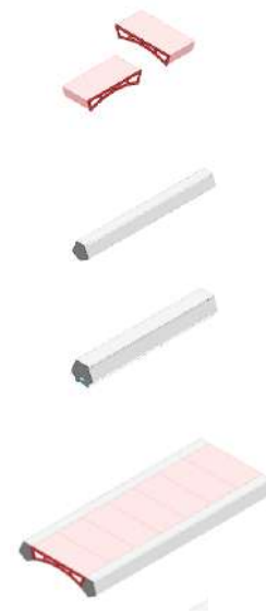
Hollow pre-cast jack-arch module, RCC pre-cast joist & assembly
